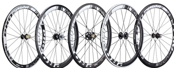
**High Profile Rims:** Fast and flat – when you need to keep up a high speed on flat roads, aerodynamics are the most important factor. Rim heights of 90mm are common for rear wheels – especially on outdoor Time Trial and Triathlon courses. High profile rims are typically a bit heavier and a heavier rim tends to preserve momentum better on a long, flat course.
