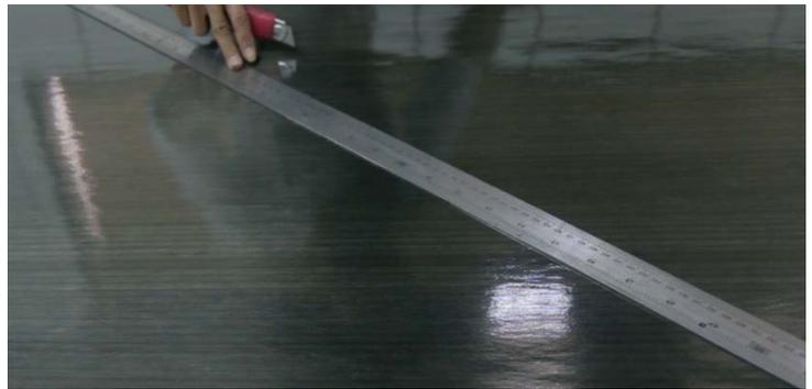
Factory sealed pre-preg UD fiber on the cutting table
