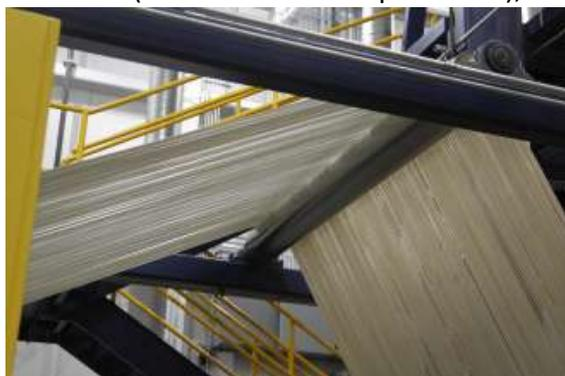
Raw PAN fibers start the process in a giant white sheet on rollers.
