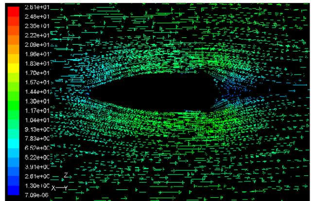
Fig. 9 – CFD model of at 50km/h rotation and wind speed showing small area of trailing edge separation (blue)
