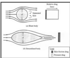
The trailing edge is the edge where air comes back together. Theoretical models often use very sharp points, but carbon doesn't like sharp angles, so in actual product, a slightly rounded trailing edge gives the best results for strength. A cylindrical airfoil has a rounded trailing edge and creates a lot of turbulence.
